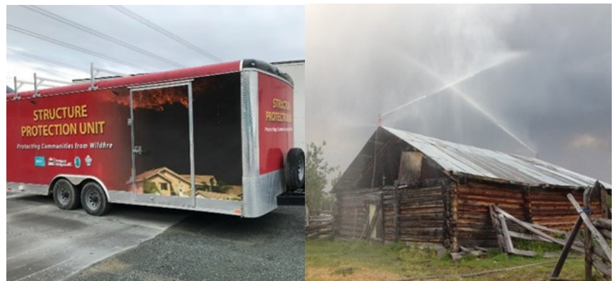
Structural Protection Unit Trailer and sprinkler system deployed on a structure.
